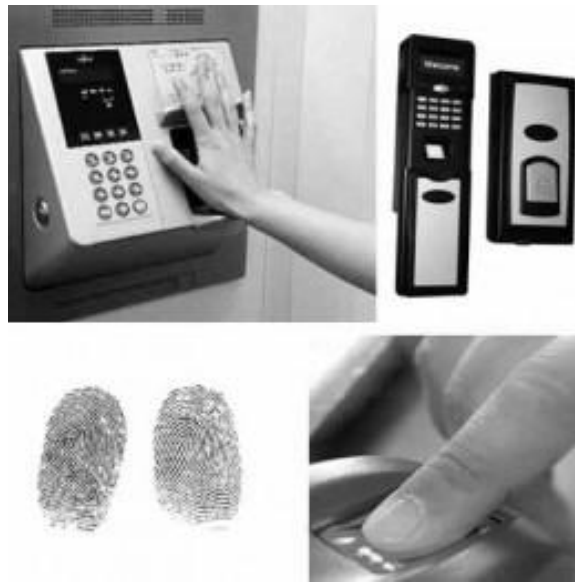
[Fig. 6] Sample employee attendance monitoring system through fingerprint and hand recognition and password based system[11]
